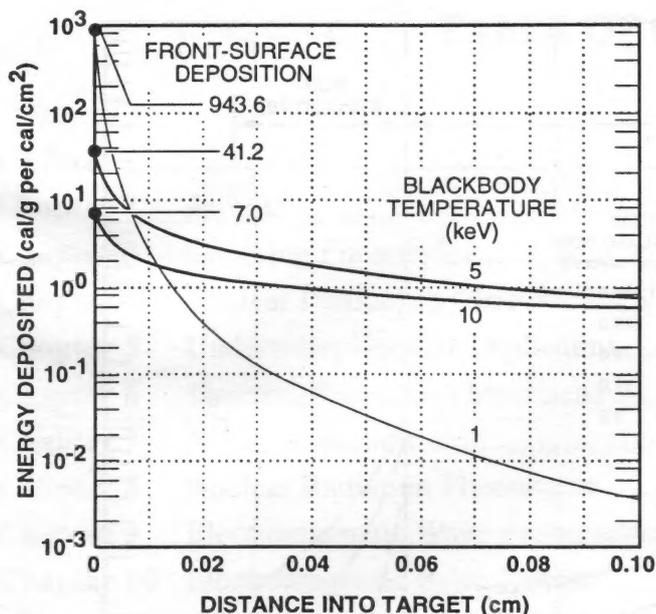
Figure 7.8. ANISN Deposition Profile for Aluminum at Blackbody Temperatures of 1, 5, and 10 keV (Incident Fluence = 1 cal/cm<sup>2</sup>).
